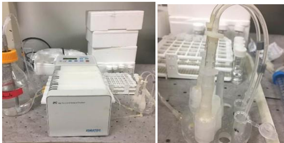
Figure 2. Experimental set-up with mini-columns (~1cm 3 ) filled with dried uranium-bearing precipitate.
