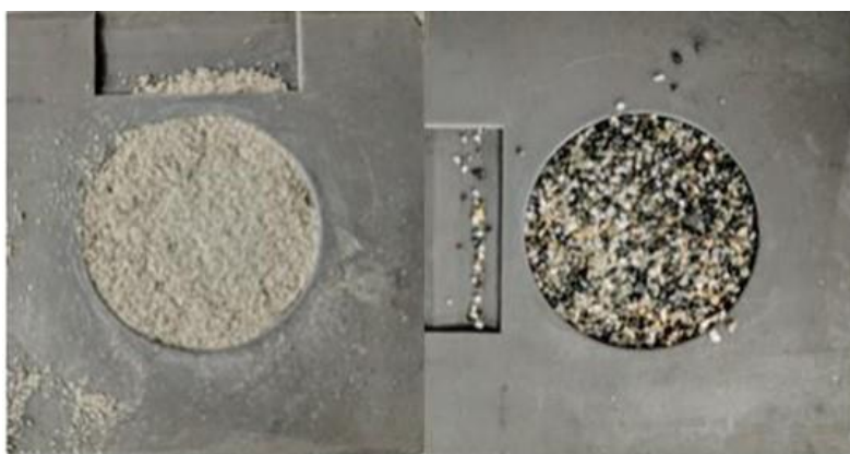
Figure 63. Example of Hanford sediment crushed (left) as opposed to not crushed (right) for XRD analysis
