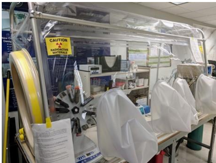
Figure 64. Anaerobic glovebox at FIU EC1227 where pertechnetate reduction experiments are currently taking place under 98% N 2 : 2% H 2 atmosphere.
