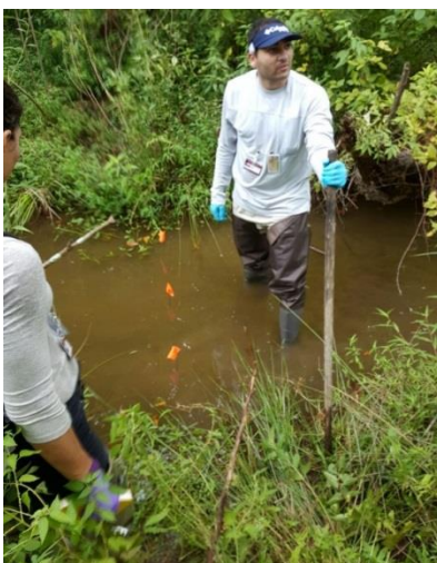
Figure 110. Flag placement across the stream width to identify measurement points.
