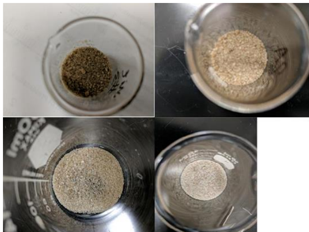
Figure 82. “Sat” acidified profile (upper left), soil after 1 cycle (7 days) contact with HNO 3 (upper right), after 3 cycles (30 days) contact with HNO 3 (lower left) and after 5 cycles (50 days) contact with HNO 3 (lower right)
